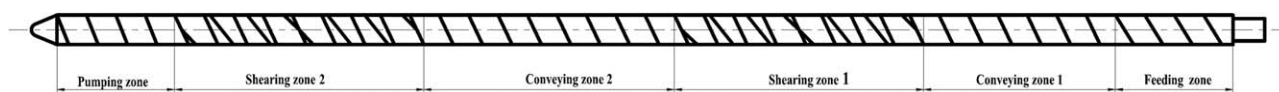
Figure 1. Schematics for screw of industrially sized single-screw extruder used in this work.
